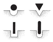
A flat file should be used for general-purpose work, a square file for enlarging rectangular holes and a round file for enlarging round holes. A half-round file can be used for dual purposes, the flat face for filing flat surfaces and the curved face for grooves.
